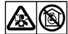
The exhaust gases are dangerous Do not use in a poorly-ventilated area
